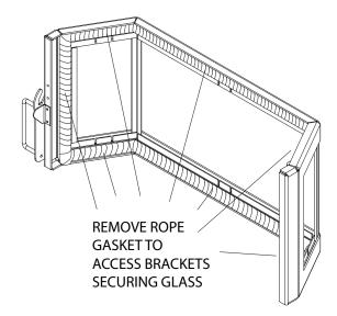
2. Remove all the nuts securing the brackets holding the glass in place.
