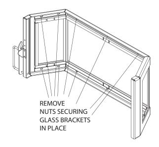
3. Once all the brackets are removed, you can disassemble and remove the glass, gaskets and vertical glass corner pieces and clean them off. Once they are cleaned, re-install the vertical glass corner pieces as shown.
