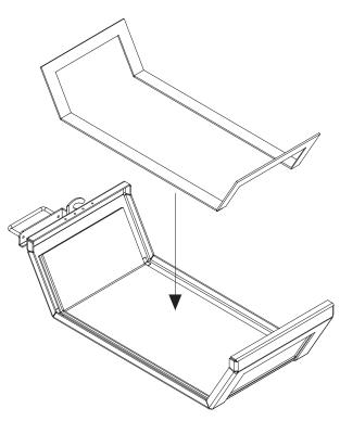
8. Once the brackets are in place and secure, re-install the rope gasket. Once the rope gasket is installed, then trim the excess glass gaskets as shown below.
